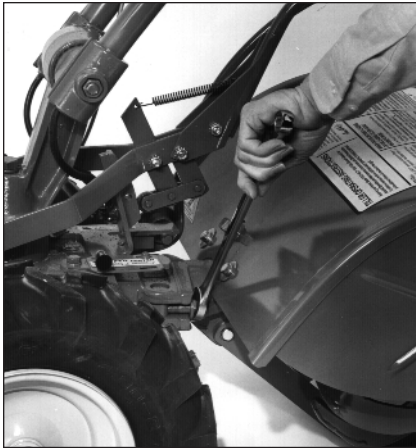
Figure 4-24: Loosening attachment swing-bolts.
